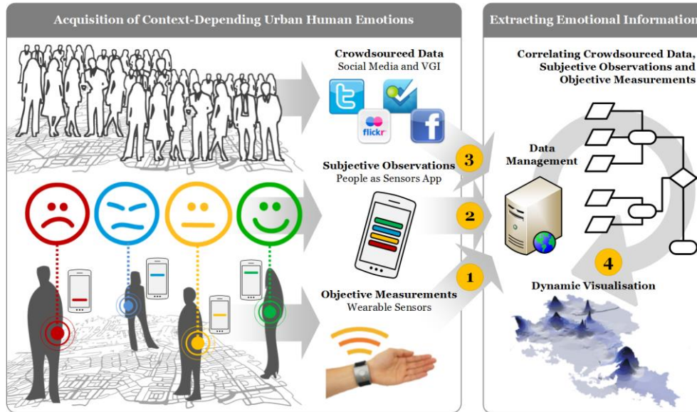
Figure 1: Urban Emotions concept: 1) emotion sensing, 2) ground-truthing using People as Sensors, 3) extraction of emotion information from VGI, 4) correlating measured and extracted emotions; plus visualisation and enrichment of urban planning processes.
