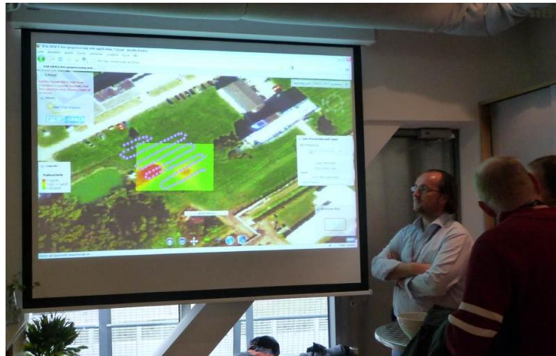
Figure 6 ‘Command and control centre’: the near real-time web-application demonstrates live Kriging interpolation of the sensor measurements (see online version for colours)
